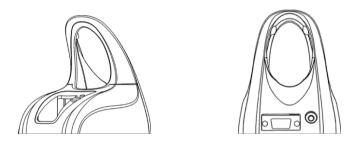
Connect the interface cable into the 15-pin connector at the back of the base. There are three types of cables available: RS232, Keyboard or USB.
