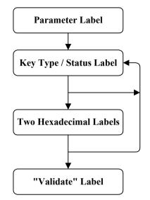
For example, to configure the Prefix Code to be "AB", the "Prefix Code" label is first read, and then the hexadecimal digit labels "4", "1", "4", and "2" are read, and finally, the "Validate" label to complete the setting.
