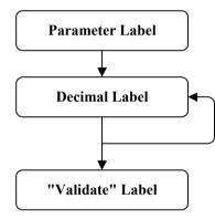
For example, to configure the Inter-Character Delay to be 15 ms, the "Inter-Character Delay" label is first read, and then the decimal digit labels "1" and "5", and finally, the "Validate" label to complete the setting.
