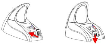
Insert the battery in front of the base to charge your battery with the power adaptor connected. When charging, the base charging LED will be RED. When the battery is fully charged, around 4 hours from completely empty battery, the LED will be solid GREEN.
