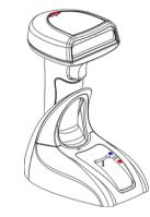
Place the scanner (with the battery inserted) on the base to charge your scanner. When charging, the scanner LED will flash RED. When the battery is fully charged, around 4 hours from completely empty battery, the LED stays on solid RED.
