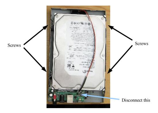
6. Gently, and very slowly, slide the drive forward away from the SATA connector. The connector is soldered onto the board, so if it breaks you'll need to re-solder a lot of tiny connections. Remember to put the four screws back in when you reassemble the drive, otherwise the only thing holding it in will be the SATA connector and it will probably break from the stress!
